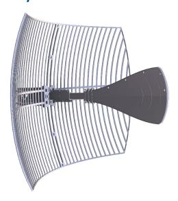
The Powertec Wideband Parabolic Grid Antenna is designed to provide high gain across the entire 3G, 4G, and 5G bands on all cellular networks throughout the Asia Pacific region. This grid antenna combines a reverse-log feedhorn with its 900 x 600 mm reflector to produce peak gains from 11.4 to 13.3 dBi on the low-band and as high as 20.8 dBi on the 4G-5G mid-band.
