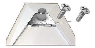
This is an optional step using M6 screws (not included) to eliminate any flex in the dish where the locking tabs click into.
